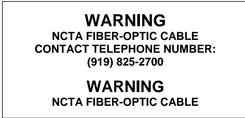
Figure 4-1. NCTA Communication Cable Identification Marker.
